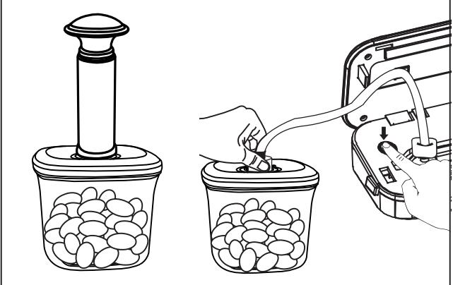
2. After closing the lid, use the vacuum pump, align the suction port and activate the vacuum pump to start vacuuming, or use it with the vacuum sealer.
