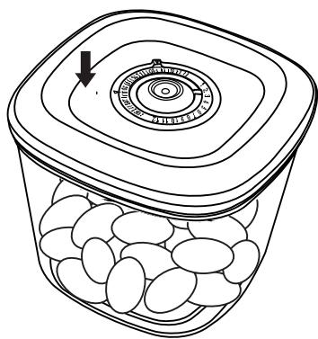
3. When the sealing cap is dented, it's finished working and reach the vacuum status, and the pointer on the time compass can be adjusted to the current date.
